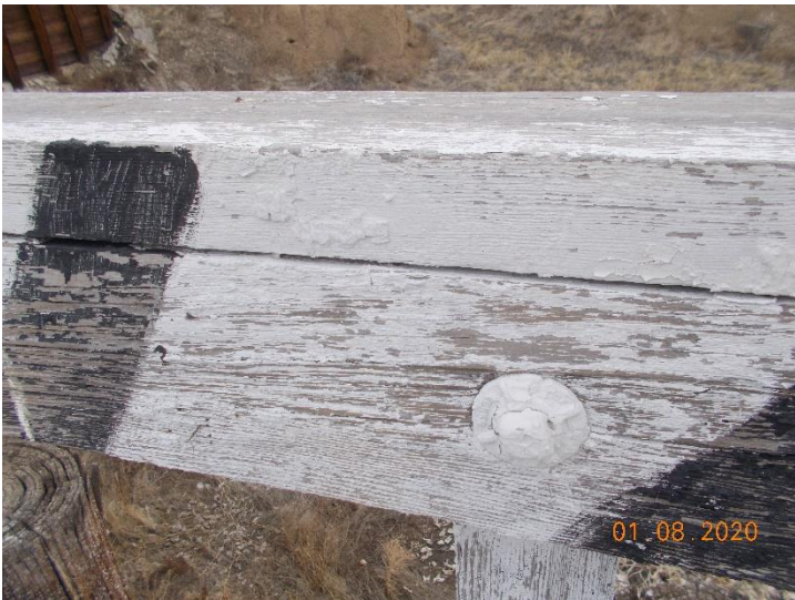
Paint sample N-21-C-LP01. The white paint on wood is considered lead-containing paint.
