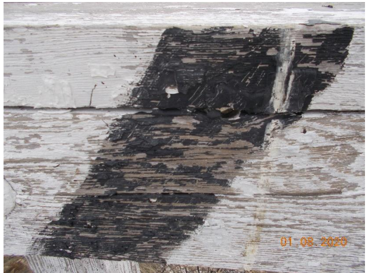
Paint sample N-21-C-LP02. The black paint on wood is considered lead-based paint.
